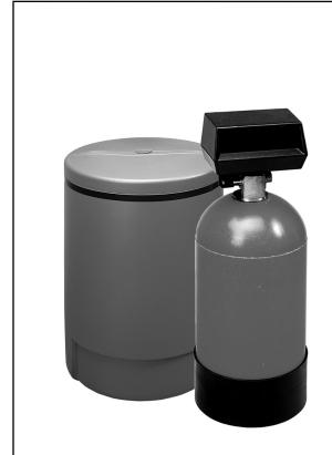
HWS050 Rated for 16,000 grains per tank, 5 gpm (18.9 lpm) service flow, 150°F (65.6°C)
